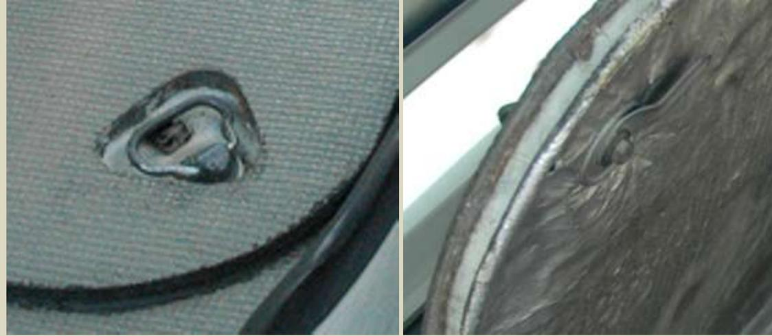
Above: Early-1962's had the engine trapdoor metal painted to match the body color (but all other years were painted black). And the 1962-63's aluminum foil-type material was wrapped around the metal edge.
