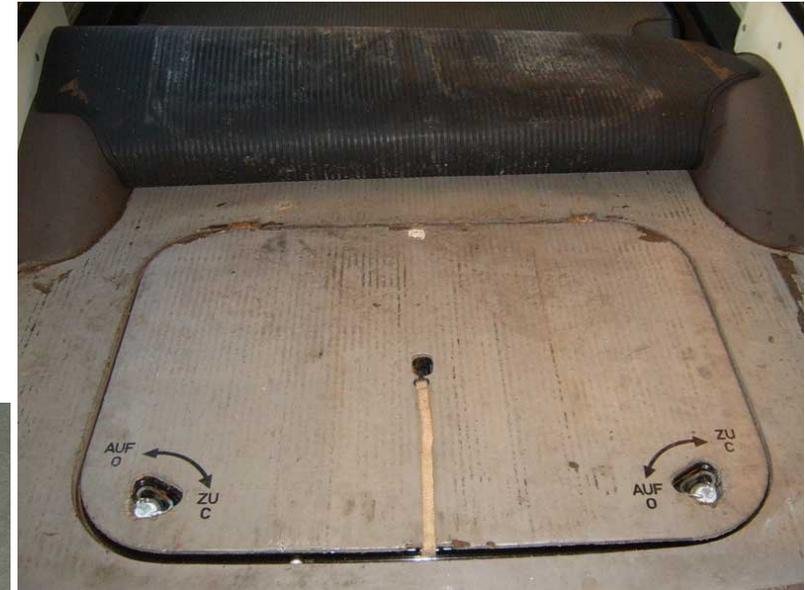
RIGHT: Late T34s from 1967-69 featured a trapdoor with OPEN & CLOSED printed on the lid. Also, the trapdoor & surrounding insulation surfaces were level, allowing the liner covering it to lay flat in the rear compartment.
