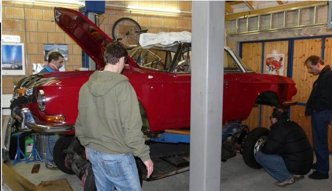
It was around midnight when Roland pulled-up the carpet behind the back seat in the area underneath the rear window shelf (above) and discovered two long bolts that had to be removed! Finally the body was apart from the chassis that same night (upper right). Philip was relieved to have solved that problem with the help of his friends and also happy to see only minor rust on the body to be repaired.
