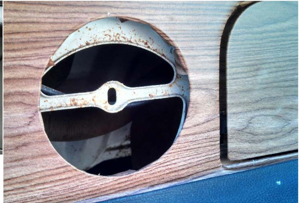
When installing the late style, fitted to T34s from 1967-69, the mounting bracket was already built-in (above), stamped with the new dash design along with the redesigned rectangular radio area. This allowed the speaker cover to be more quickly installed by simply screwing the machine screw into the cover.
