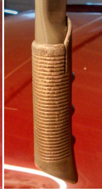
Apply two coats of primer and allow to dry overnight. Then apply two coats of the Anthracite spray paint from Wolfsburg West (Southern California USA) and allow to dry overnight. For a protective shine, spray one coat of clear, as the e-brake handle gets nicked by seat belt buckles & rubbed by forearms when driving.
